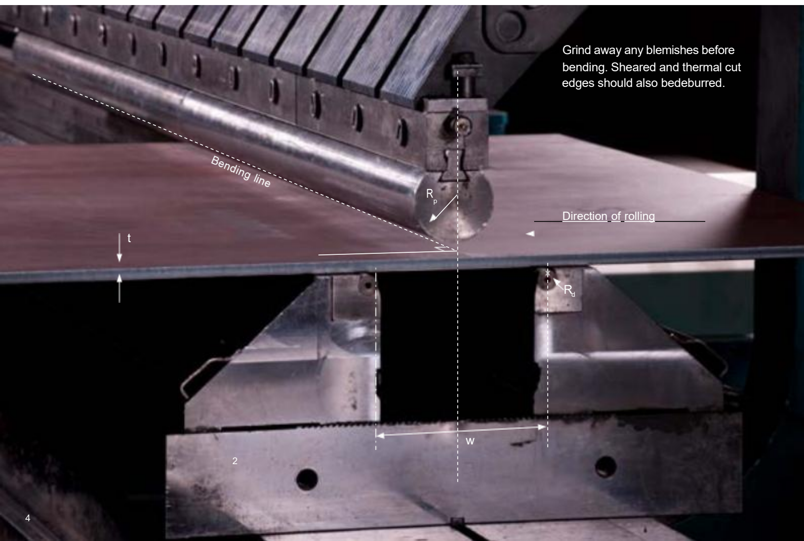
FIGURE 1 Bending transverse to the direction of rolling.
